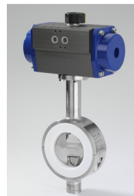
Wafer SS316L (1.4435) PTFE/PFA, pneum. actuator
